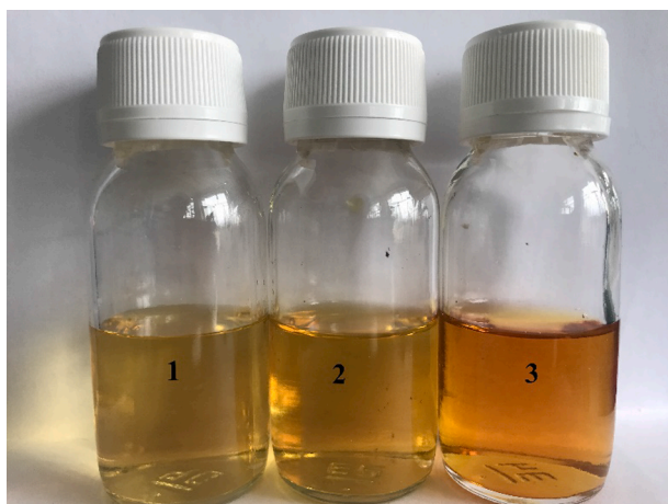
Fig. 2. Solutions of iodine (1) and their complexes with 50 kDa POZ (2) and 44–54 kDa PVP (3). Concentration of iodine in these solutions was 0.004 w/v % with 1.2 w/v % KI. Concentrations of POZ and PVP were 0.0078 w/v % and 0.0175 w/v %, respectively.
